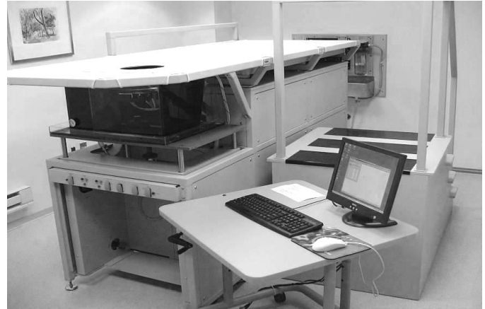
Fig 6. An ultrasound tomography scanner located at the Karmanos Cancer Institute in Detroit, MI, USA.
