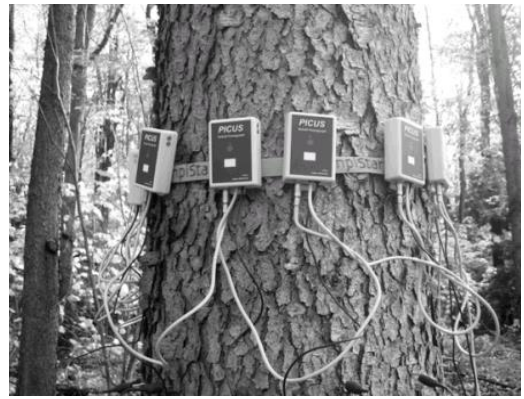
Fig 2. An array of sensors is used to perform transmission tomography for imaging the inside of a tree trunk. This commercial product is branded as PiCUS Tomography, Argus Electronic, Rostock, Germany.
