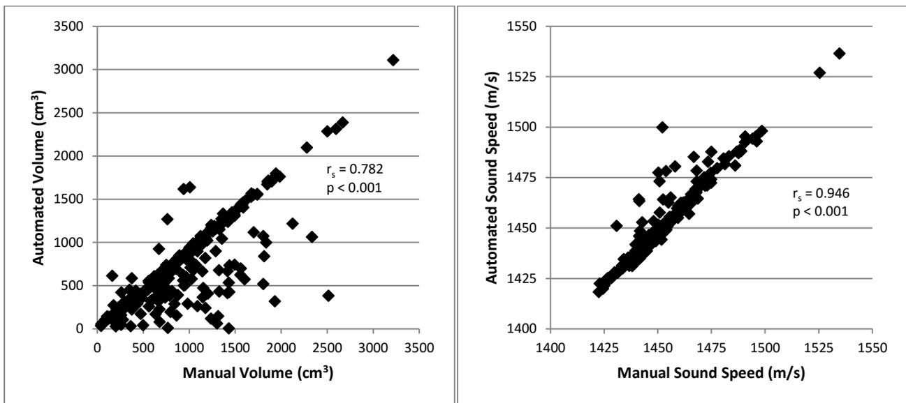
**Figure 2** – (Left) Plot of the measured volume of the automated masks versus the volume of the manual masks. (Right) Plot of the mean sound speed measured using the automated masks versus the mean sound speed measured using the manual masks. The noise in the sound speed plot is lower than for the volume plot indicating that measured sound speed is less sensitive to changes in volume.
