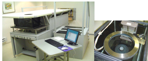
Figure 1. Experimental setup (left) and close-up of ultrasound ring transducer.
