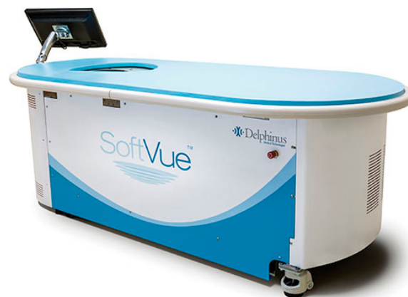
Figure 1. The SoftVue BTUS unit uses a prone water bath and ring array to scan in the coronal plane.
