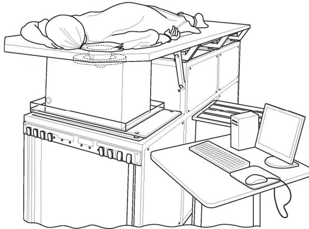
**Figure 1:** The UST clinical prototype. A patient lies in the prone position such that the breast is suspended inside a water tank that contains the ultrasound sensor. The water acts as a coupling medium to ensure that the acoustic waves can penetrate the breast efficiently.
