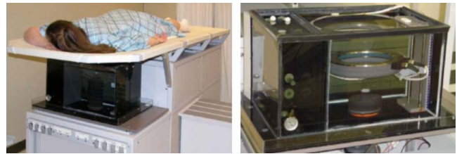
FIG. 1. The patient setup and clinical prototype of the CURE device. Left: Prone patient positioning for the CURE scan. Right: Close-up of the imaging tank showing the transducer ring affixed to a mechanical arm that steps the ring down while imaging the entire breast volume.
