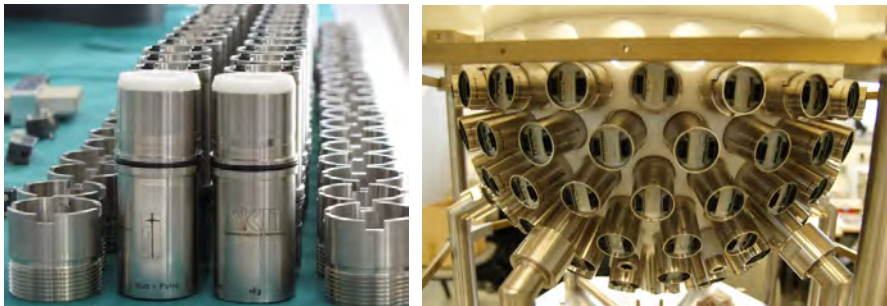
Figure 1: Left: USCT 2.0 TAS systems transducers before assembly in the final system. Right: Semi-ellipsoidal aperture of USCT 2.0
