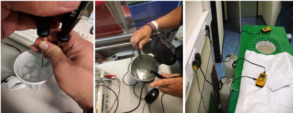
Figure 9: left and middle: calibration of Greisinger temperature measurement probes, right: setup for measuring the heat-up of the 3D USCT 2.0 and air temperature for improved calibration
