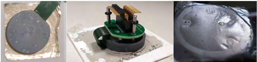
Figure 21: Left: Holes of the PVC substrate filled with PU-tungsten composite backing material. The backing is only applied behind the sensor elements. The backing and flex print are glued onto the tin foil matching. Middle: Pins align the back end of the PCB to fit in the casing later. Right: Tin foil matching layer after application.
