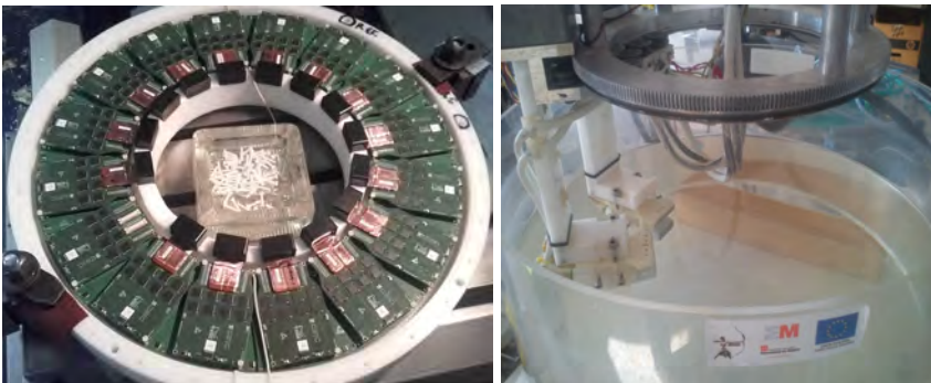
Figure 1: (left) Ring transducer of the MUBI system (right) proof of concept with moving arrays.
